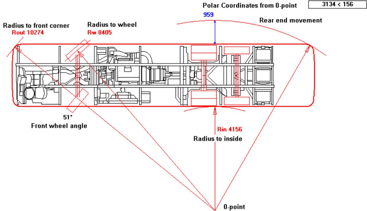
This Combo box on the upper corner of the screen gives the possibility to choose **R out**. The program calculates then corresponding front wheel angle and **R in** and Rear end movement
