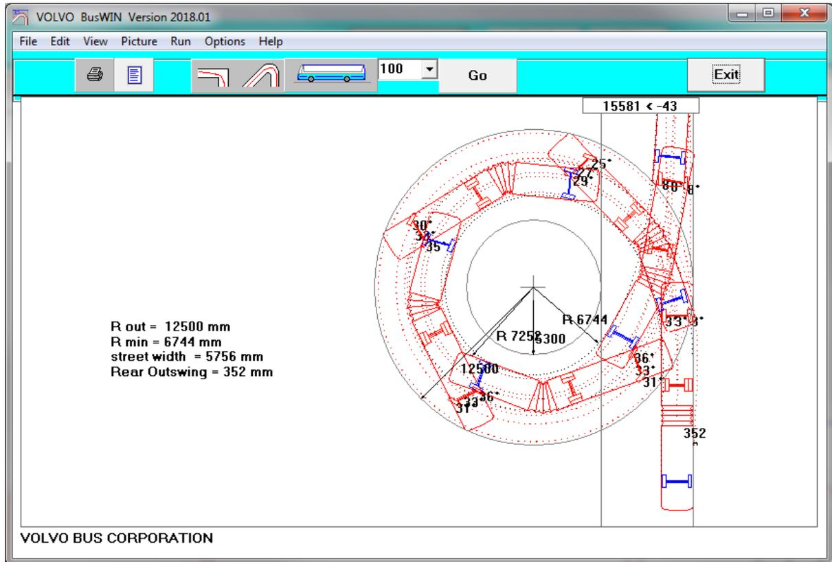
Turning in 360 deg arc. The vehicle comes direct, tangential to the circle, drives full circle, 360 degrees, following the outer side of the circle and then drives tangential out. The default radius is 12.5 m. The Program calculates the minimum radius Rin to the vehicle inside.
