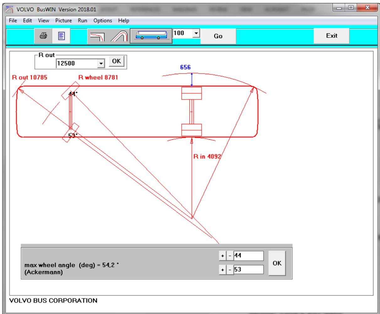
Calculating R out ( Radius to the front corner of the vehicle ) and R wheel ( Radius to the center of front wheel ) with chosen steering angle. From the text boxes below you can adjust the steering angles for inner & outer wheels separately. The default values comes from chassis data. You can also edit the values by using "+" and "-" buttons.
