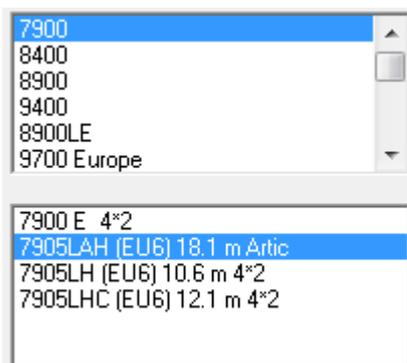
From the first listbox below you can choose bus chassis model group. As last choice in the list you can find a group named xxx, this means default chassis that can be used for simulating different new types.
